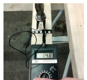
Fig. 3: Wood moisture measurement after leak-tightness test
