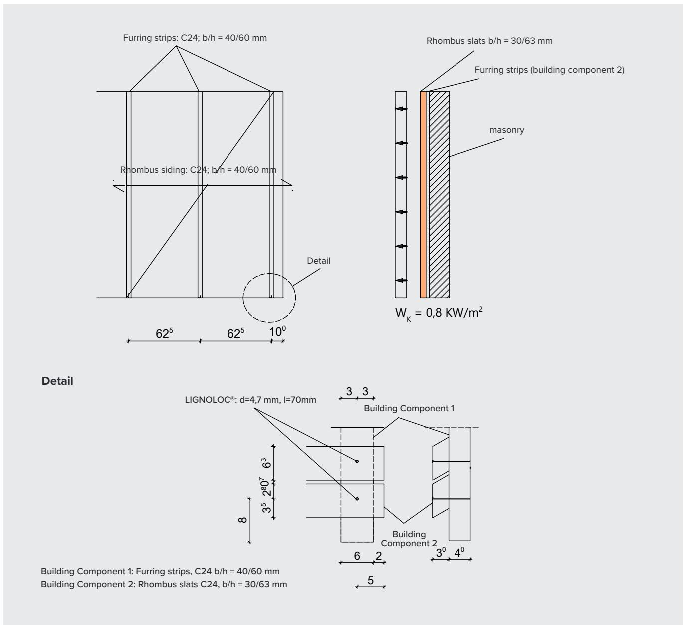
An analysis of the entire building resulted in a governing characteristic wind uplift action of 0.8  $\text{kN/m}^2$ . For the rhombus profile slats, an average density of  $\rho_{\text{mean, Timber}} = 4,2 \text{ kN/m}^2$  can be assumed.
