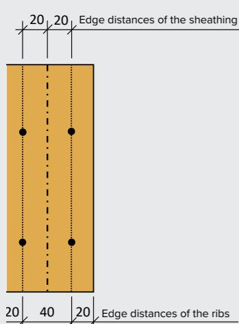
Have the minimum fastener spacing requirements in the studs been met?
