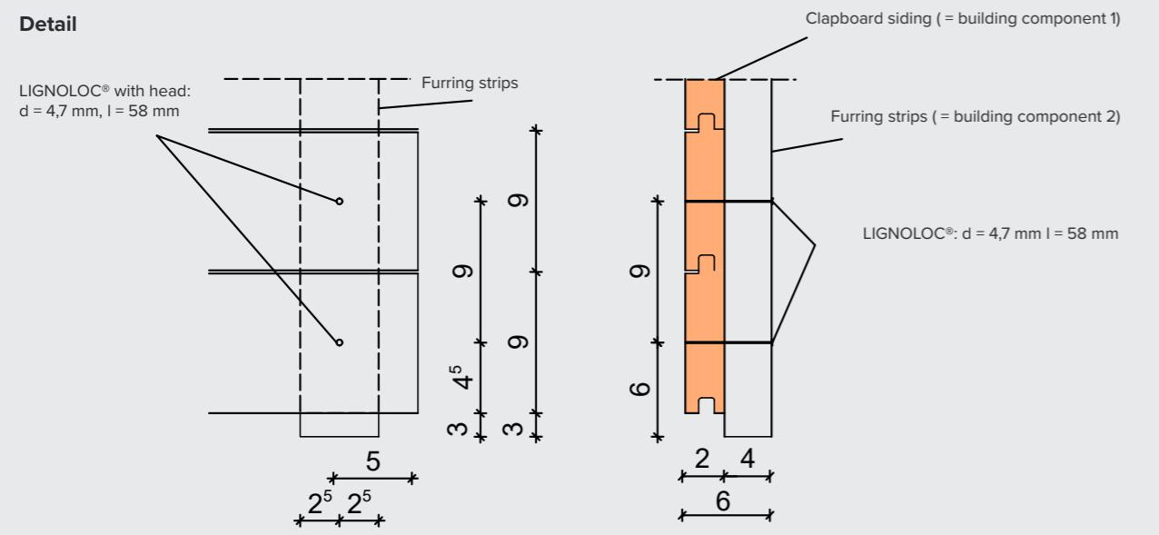
An analysis of the entire building resulted in a governing characteristic wind uplift load of  $0.8 \text{ kN/m}^2$ . For the clapboard siding, an average unit weight of  $\rho_{\text{mean, Timber}} = 4,2 \text{ kN/m}^3$  can be assumed.
