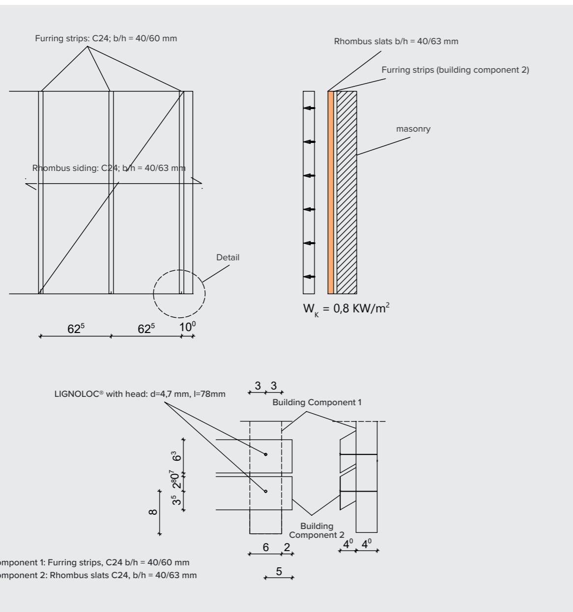
An analysis of the entire building resulted in a governing characteristic wind uplift action of 0.8  $\text{kN/m}^2$ . For the rhombus profile slats, an average density of  $\rho_{\text{mean, Timber}} = 4,2 \text{ kN/m}^3$  can be assumed.
